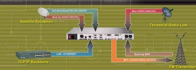
At each transmitter site, Shark receives analog and/or digital stereo feeds and digitally combines them into a Composite signal. RDS data are added at the same time, from integrated digital RDS coder. Overall MPX output then feeds one or more Exciters for FM broadcasting.
