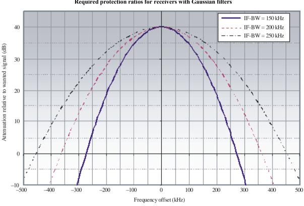
FIGURE 2 Required protection ratios for receivers with Gaussian filters
