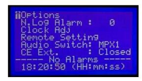
By operating the encoder knob you can move the cursor to the needed setting.
