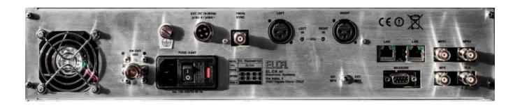
STEREO SECTION: INT. MPX Internal Stereo Coder is working (option A) EXT. MPX External MPX Input is working
