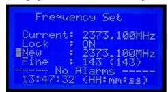
By operating the knob as before explained you can select a different frequency from the one currently set, obviously provided that it falls within the allowed range: by moving the cursor and clicking on the *New* setting, you can directly change the frequency value in 1kHz, 10kHz steps, etc. At the end of the operation, the caption "pres " is displayed. To switch the equipment to the new frequency just briefly press the knob.
