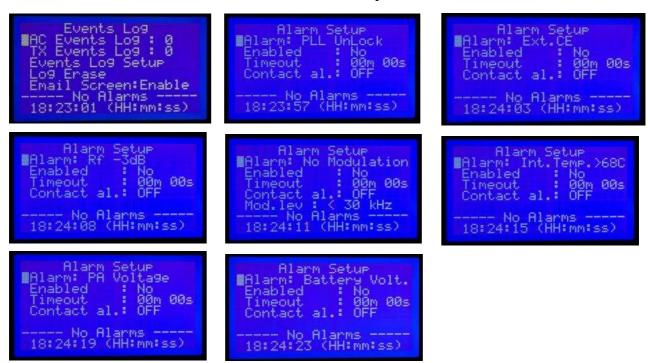
The first two lines of the submenu, *AC Events Log* and *TX Events Log*, are used to check the alarms currently stored in memory: for each of them the date, time and type of the alarm is recorded, along with the date and time in which the system returned to its normal operating condition. The equipment can store in memory up to 100 alarm events. When this value is reached, a FIFO policy is used which deletes the oldest alarm and places the newest one at the top of the stack.
