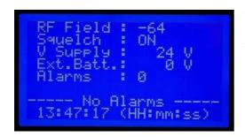
This setting shows the value of the signal level received at the antenna input.
