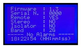
By accessing this menu page you can check a number of available options: **Remote-Stereo-Insulator**, the installed **Firmware** release and the equipment **Serial N.**, which is particularly important in case the REMOTE option is installed, because it enables the user to set the parameters when in **Remote** mode.
