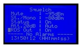
In the page selected by clicking on the *Squelch* setting, you can check the current levels for several parameters and set new values. Two of them, *St./Mono* and *RDS out*, are only available if Option A is installed.
