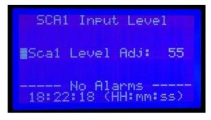
Here you can check the audio level and change it to the needed value: all input levels between -1dBm and + 13dBm are allowed.
