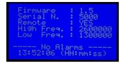
By accessing this menu page you can check a number of available options, the installed software release and the equipment Serial Number, which is particularly important in case the REMOTE option is installed.
