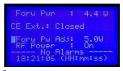
In this page you can set the output power in 0.1W steps and turn the output power off by software putting the TX in stand-by mode.
