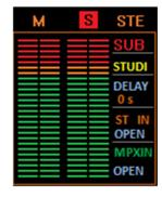
In the lower left, in correspondence to the symbols that identify the input signals (M = Main, S = Sub), shows the levels of the Stereo input channels.
