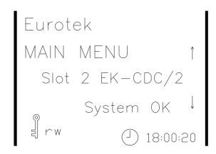
Pushing the enter key (EK-MFR/1 manual, *board panel description*) it is possible to explore the EK-CDC/2 menu. We suppose to set the Video in variable. To do this it is necessary to run (using the Explorer menu and display mode keys (EK-MFR/1 manual, *front panel description*) until the Port Set menu as the next figure shows:
