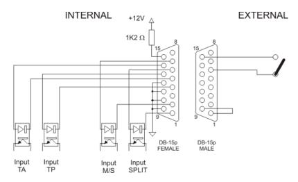
Tie together pin 1 and 9 and shortcut pin 15 and pin 6 via an external switch.
