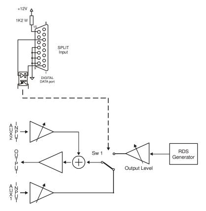
The output will contain the external signal applied to AUX 1 connector. The internal RDS generator is disconnected.
