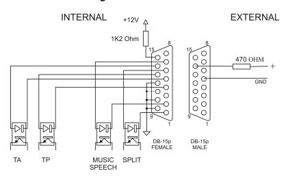
Apply an external TTL signal <u>through a 470 Ohm</u> carbon resistor to the TA photodiode (pins 14 and 5). Max current allowed: 10 mA. Nominal: 5 mA
