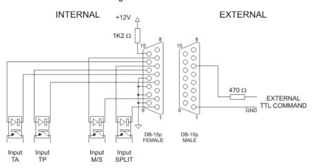
Apply an external TTL signal <u>through a 470 Ohm</u> carbon resistor to the SPLIT photodiode (pins 6 and 1). Max current allowed: 10 mA. Nominal: 5 mA
