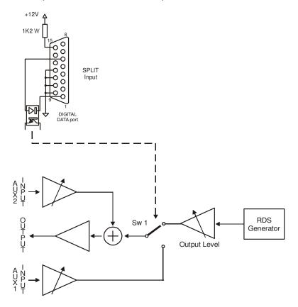
The output will contain the RDS signal generated by the coder. The RDS signal will pass through the SW 1 switch.
