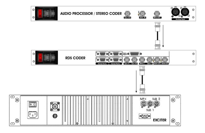
In the loop-through mode, the output of the stereo generator is directly cabled at the AUX 1 input of RDS encoder. The RDS output of the encoder will be then connected to the normal composite/Mpx input of the FM exciter.
