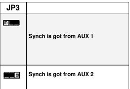
RDS synch reference is get by default by internal source reference. Use the Pc Control software mask (see paragraph 17.3) to enable External Synch reference.
